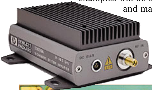
The HP 83017A microwave system amplifier achieves 0.5–26.5 GHz bandwidth by incorporating the HP TC702 GaAs MESFET TWA IC.
